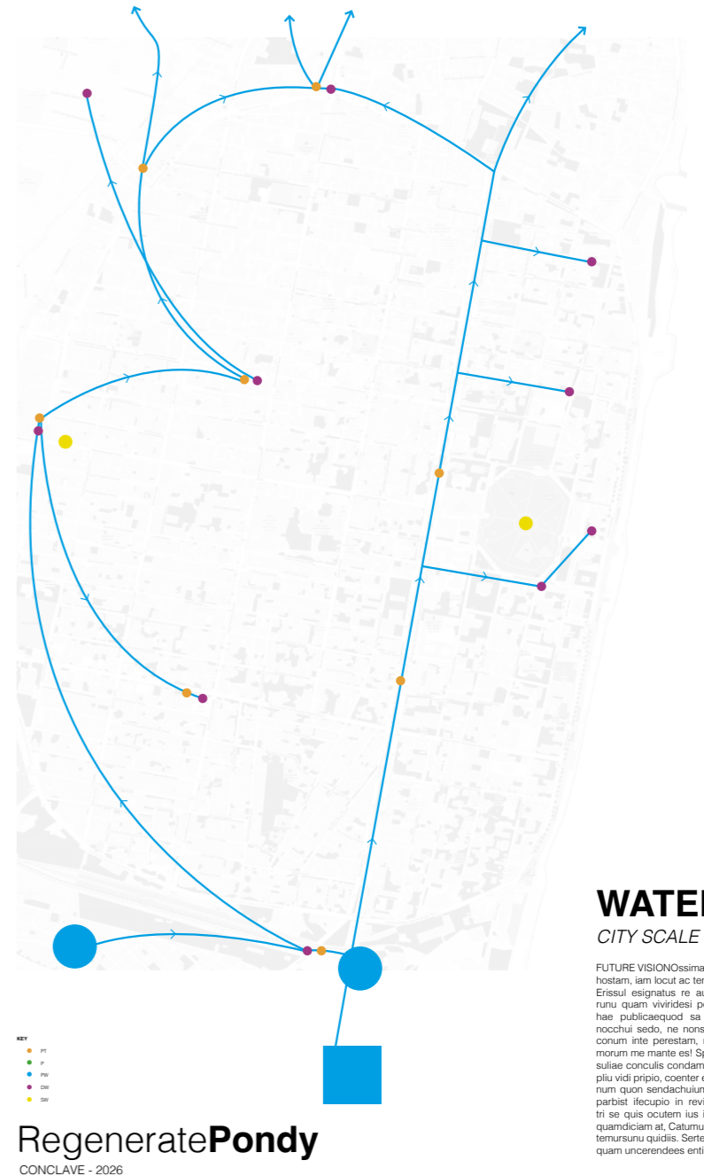
Figure 55. Vision at the city scale for the water system (in which: PT – Purification tank, DW – Drinking water, SW – Sewage, PW – Purified water)
